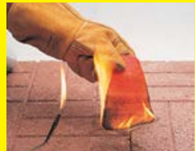
Ordinary foam lining ignites after only a two second exposure to flame.
