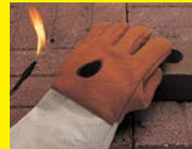
COMFOflex ® lining does not ignite after a four second exposure to open flame
