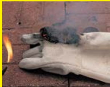
Ordinary cotton lining continues to smoulder after a two second exposure to flame.
