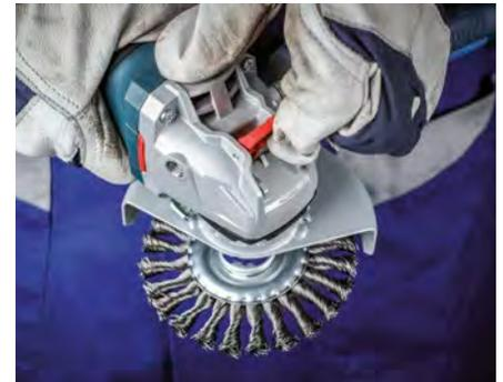
Release the brush by using the lever.
