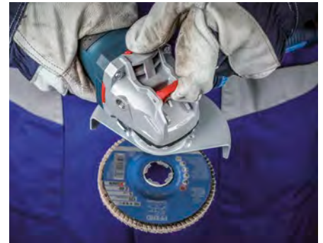
Release the disc by using the lever.
