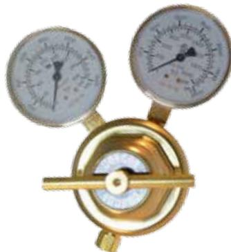
This unique regulator can be used with either **LIQUID OXYGEN OR HIGH PRESSURE CYLINDERS**. High volume regulator has 1/2" inlet and outlet ports. Regulator is available as either a manifold regulator (as pictured) or with a CGA 540 nut and nipple for high pressure cylinders.
