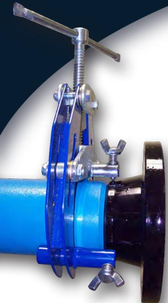
Every H&M Easy-Fit Pipe Clamp provides quick precision fit-up of flanges, fittings and pipe-to-pipe alignment. The Easy-Fit Clamps are manufactured using double-walled steel plate and are lightweight for all overhead work. They feature a T-handle which slides back and forth for easy positioning in tight locations.
