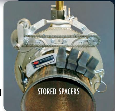
In the past 12 spacers were required. The saddle of each H&M machine and the four cuboids allow four specific pipe sizes to be cut. Each side of every cuboid spacer is clearly stamped to ensure cutting the correct pipe size. When not in use the cuboid spacers are securely housed on the back of the saddle. It's a no-lose proposition in time-saving productivity!
