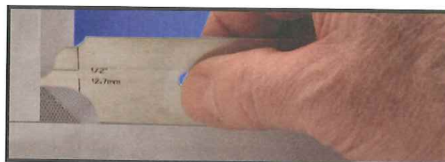
CHECKING FILLET LEG SIZE
