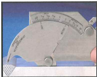
Excess Weld Metal
