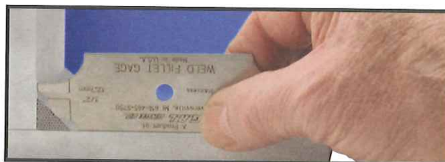
CHECKING FILLET THROAT SIZE
