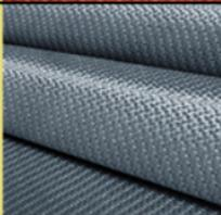
17 oz., Silver gray or red, Silicone coated Fiberglass. Light duty, 1000°F melt temperature, vertical plane protection only, .022" thick. Sizes 40" or 60" wide, 50 yard rolls, custom blankets.
