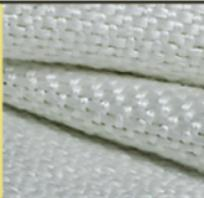
18 oz. White Fiberglass, or Heat treated tan color. No Coating. Light duty, 1000°F (540 C) melt temperature, sparks, vertical plane protection only, .03" thick. Sizes 40", 60" or 72" wide 50 yard rolls, 3'\*3, 6'\*6', 6'\*8', 8'\*8', 10'x10', custom blankets
